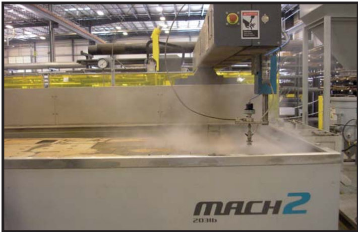
The Flow Mach 2 waterjet can cut metal materials, such as this chromium carbide, up to 250mm or 10" thick.
