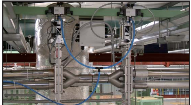
Vortex Wye Line Diverters allow the vacuum transfer of loose leaf tea from a choice of two sources to two destinations.
