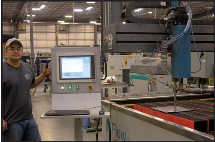
Abe Horning, Waterjet Operator, loads the computer file for the waterjet to cut a rubber seal. The special application is supported by the red waterjet bricks.
