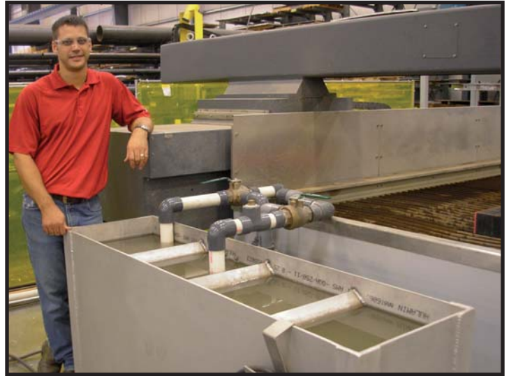
Cory Wellbrock, Fabrication/Weld Supervisor, showcases the water tank that employees designed and fabricated to recycle the water from the waterjet.
